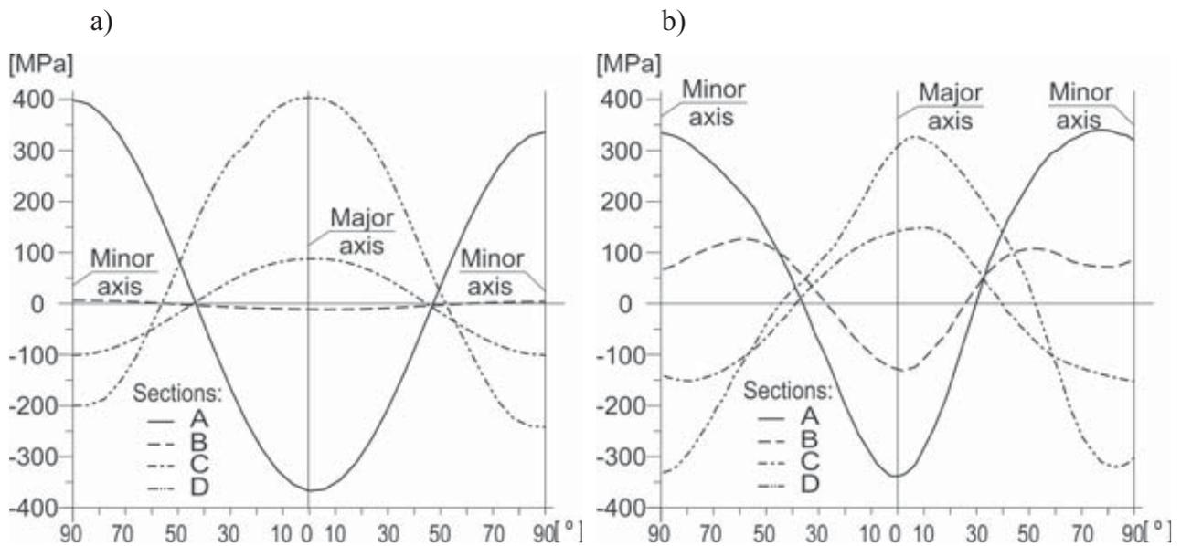
Fig. 3. Longitudinal stresses  $\sigma_2$  in specific sections of the conical part of the flexspline loaded with a torque moment of  $T_2=150$  N·m: a) determined by means of FEM b) determined by means of the extensometer method
