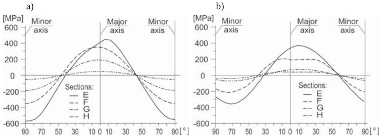
Fig. 4. Circumferential stresses  $\sigma_t$  in specific sections of the cylindrical part of the flexspline loaded with a torque moment of  $T_2=150 \text{ N}\cdot\text{m}$ : a) determined by means of FEM b) determined by means of the extensometer method
