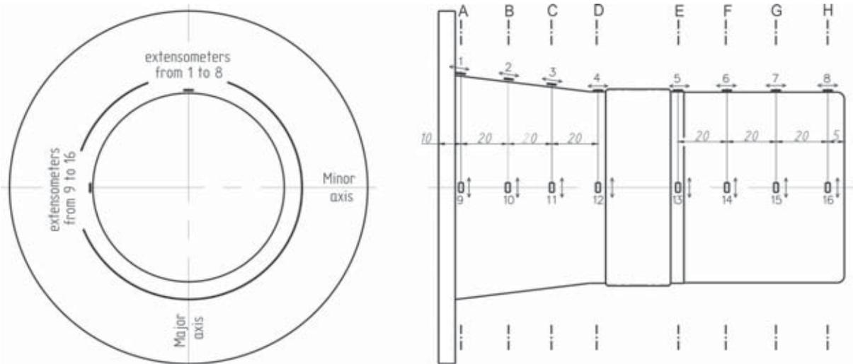
Fig. 1. A diagram of extensometers and measuring sections distribution on the flexspline. Marking: from 1-16 extensometers; A - H measuring sections
