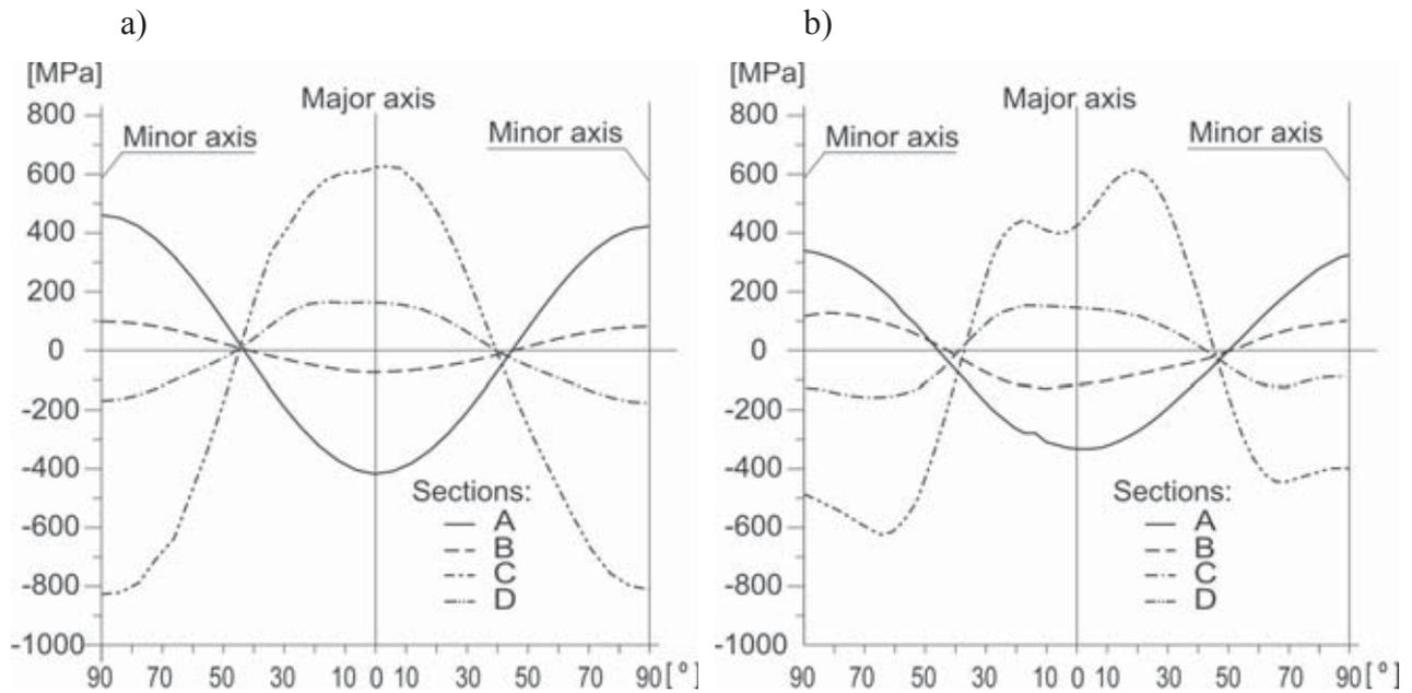
Fig. 2. Circumferential stresses  $\sigma_1$  in specific sections of the conical part of the flexspline loaded with a torque moment of  $T_2=150$  Nm: a) determined by means of FEM b) determined by means of the extensometer method
