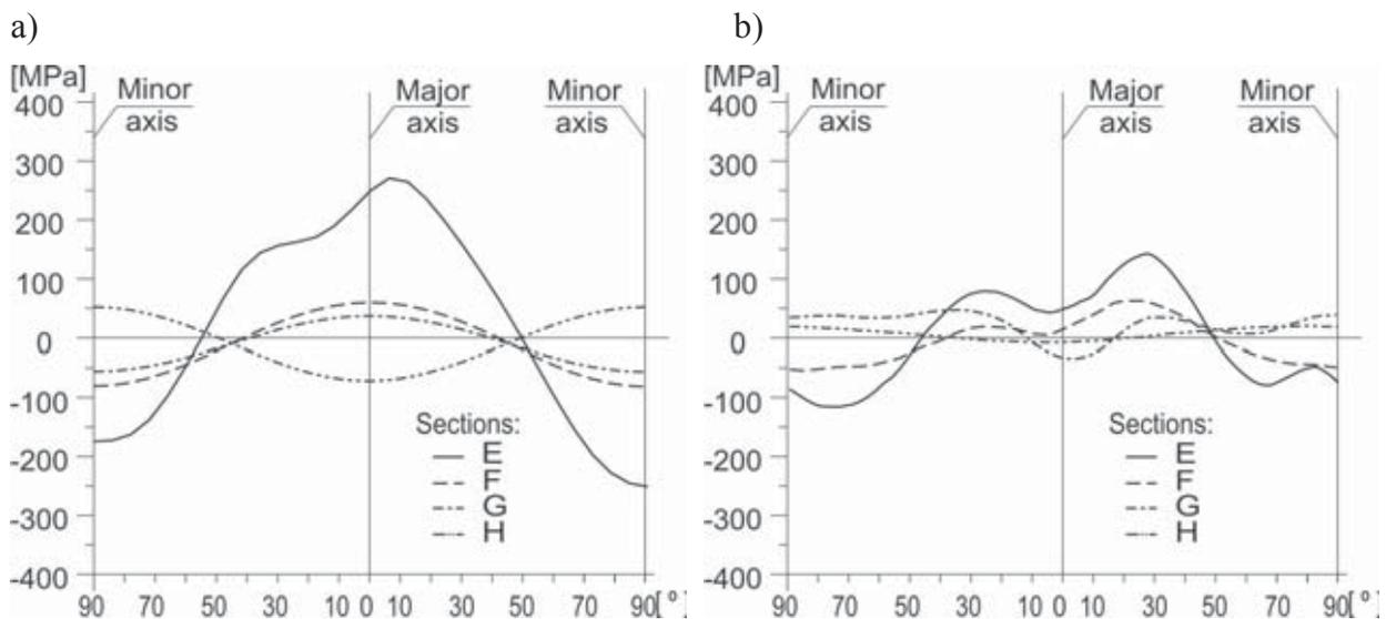
Fig. 5. Longitudinal stresses  $\sigma_l$  in specific sections of the cylindrical part of the flexspline loaded with a torque moment of  $T_2=150 \text{ N}\cdot\text{m}$ : a) determined by means of FEM b) determined by means of the extensometer method
